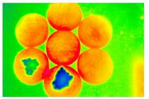
R&D testing of material absorbency and moisture permeation.
